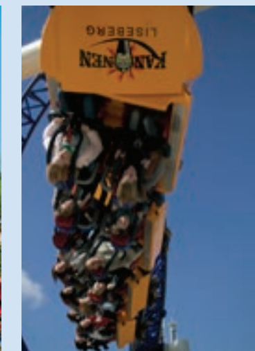
ACCELERATOR WITH INVERSIONS T.H.C.: 880 pph Height: 23 m (76 ft) Track length: 430 m (1411 ft) No. of trains: 2x16 pers.
