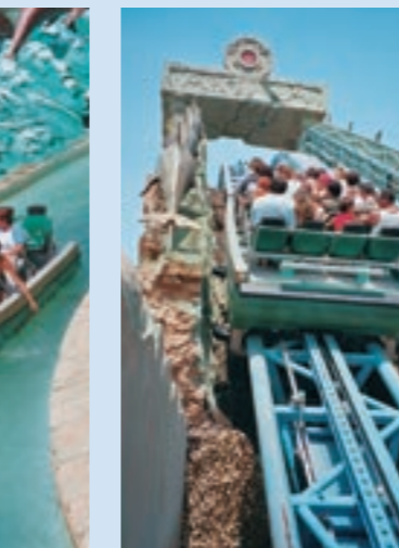
SUPER SPLASH Cable lift Lift angle: 35° Lift speed: 3.5 m/sec (115 ft/sec)
