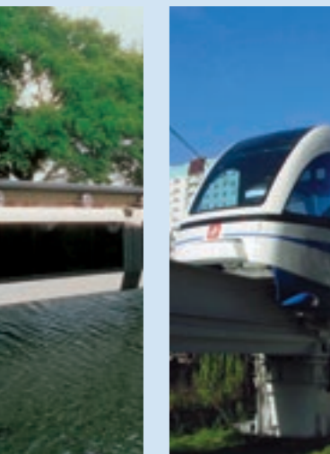
MONORAIL P30 Moscow, Russia T.H.C.: up to approx. 6000 pph Capacity per train: up to 200
