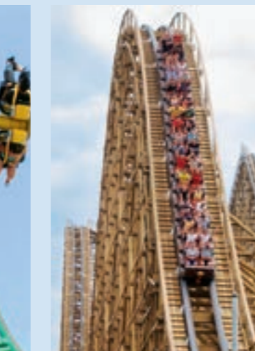
WOODEN COASTER T.H.C.: 1400 pph Height: 55 m (180 ft) Track length: 1365 m (4478 ft) New track technology
