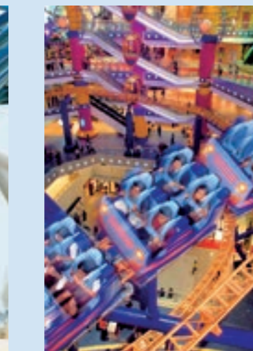
INDOOR LOOPING COASTER T.H.C.: 1000 pph Height: 30 m (100 ft) Track length: 800 m (2625 ft) No. of trains: 2x24 pers.
