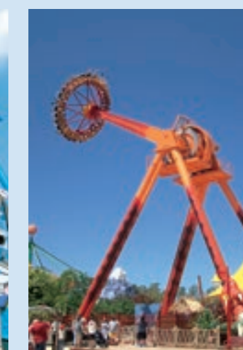
GYRO SWING Axle height: 16–31 m (53–102 ft) Swing height: 27–50 m (89–164 ft)
