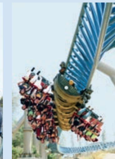
ACCELERATOR: WING RIDER T.H.C.: 1400 pph Height: 15 m (49 ft) Track length: 858 m (2815 ft) No. of trains: 3x24 pers.
