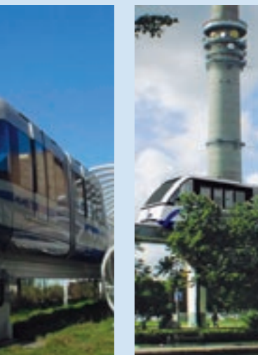
MONORAIL P30 T.H.C.: up to approx. 15000 pph Capacity per train: up to 500
